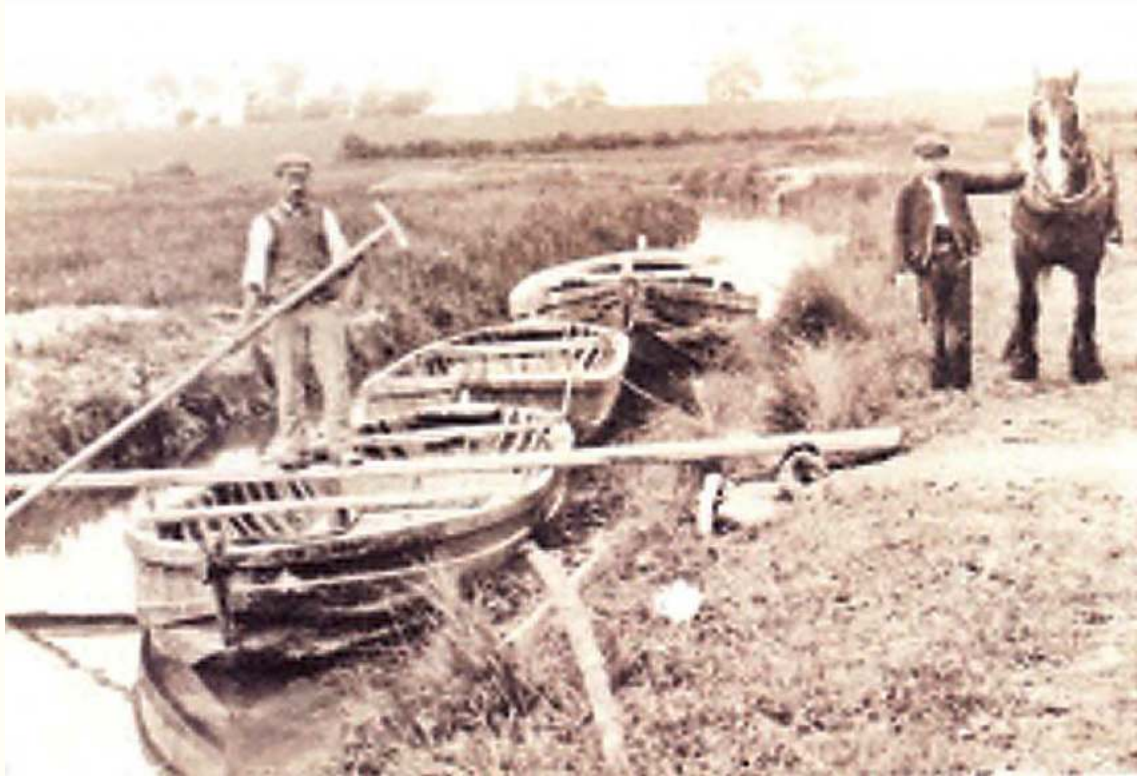
With their shallow draft and length, these Fen boats from about 1910 carried surprisingly large tonnages. Mediaeval boats using Swavesey docks were probably similar.
